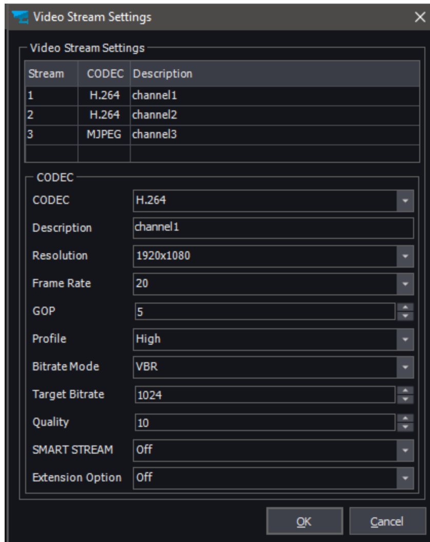
Figure 5-11: Server Settings > Camera Settings > Video Stream Settings (VISIX Gen III Cameras Only).
