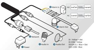
1 Power Connection Please check the voltage and current capacity of rated power carefully. PoE
