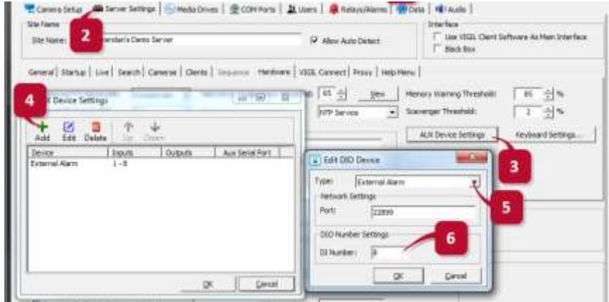
Figure 2-1: Configuring VIGIL Relays for use with ANPR Utility- Configuring AUX Settings in VIGIL Server
